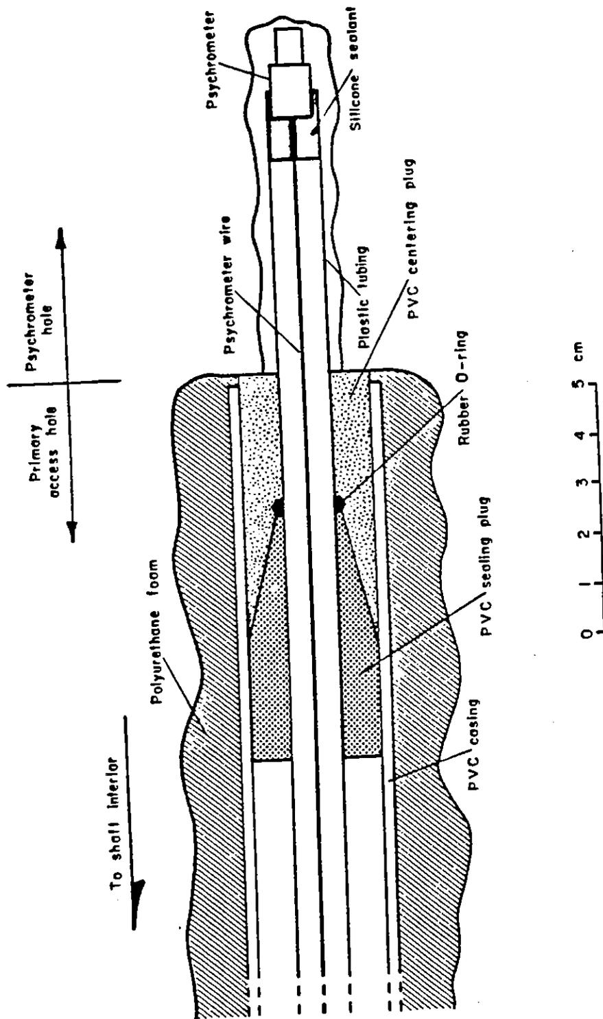
Figure 4. Schematic cross-sectional view of psychrometer installation.
