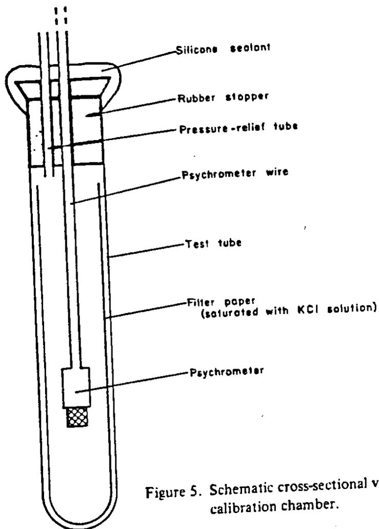
Figure 5. Schematic cross-sectional view of psychrometer calibration chamber.
