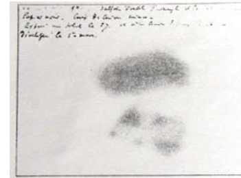
First autoradiograph indicating the discovery of radioactivity (March 1, 1896). Clear outline of a cross made of thin sheet-copper that had been placed on a photographic plate under a layer of uranium salt and kept in a dark drawer. 2
