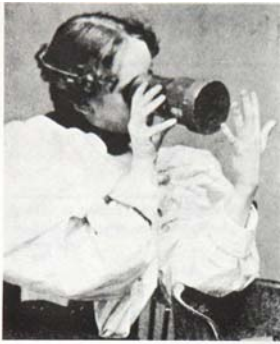
Early fluoroscope (1896). A quick way to test the x-rays being produced was to place the hand between a vacuum tube and fluorescent screen. 2
